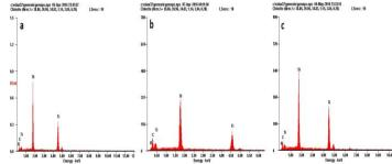
Fig.5: EDS analysis of as deposited Ti-Si-B-C coating for a) 10µm, b) 15µm and c) 20µm coating thickness
