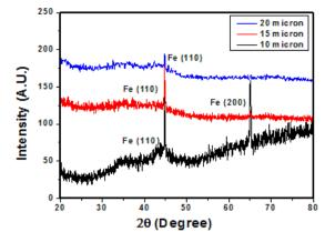
Fig.3: XRD of TiSiBC film for 10µm, 15µm and 20µm coating
